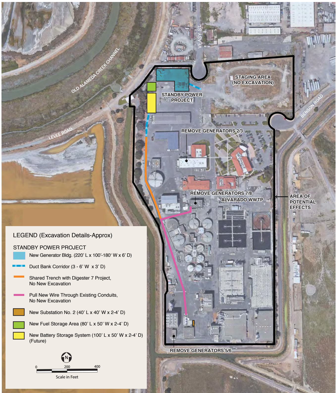
Figure 2. Construction Characteristics of Standby Power Generation System Upgrade Project
