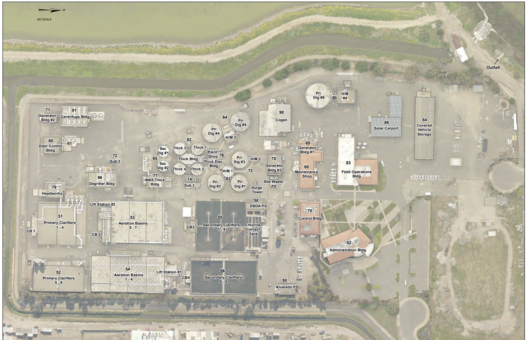
Figure 2. Existing Alvarado WWTP Site Plan
