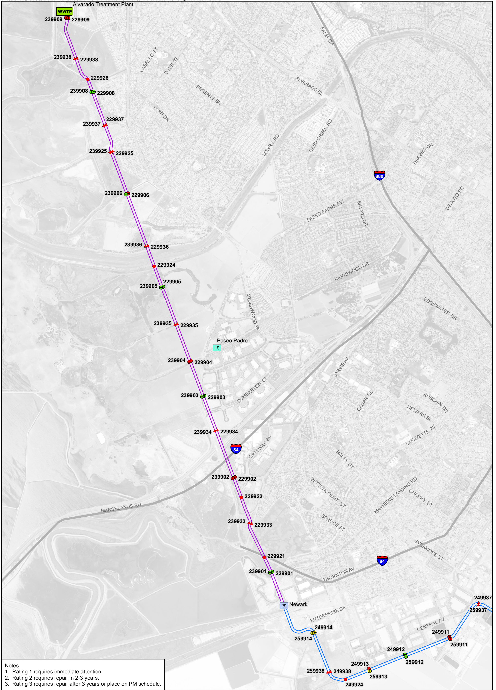
Figure 2 Newark Pump Station to Alvarado Treatment Plant Manhole Condition Ratings Union Sanitary District Force Main Manhole Corrosion Repairs
